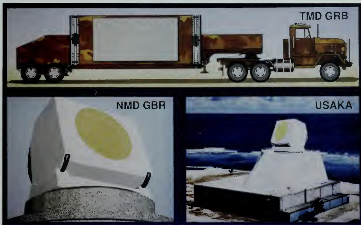
Fig. 5-19. The Ground-Based Radar Family of Radars included the truck mobile Theater Missile Defense system, the planned National Missile Defense radar and the experimental complex to be constructed at Kwajalein.
